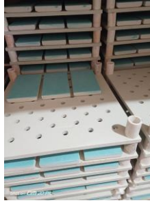
Figure 18, The tiles are cooling (Resource: Personal Archive)
