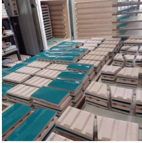
Figure 17, The tiles are in to the kiln (Resource: Personal Archive)
