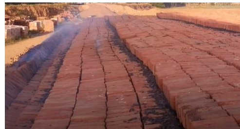
Figure 8 , The bricks and the coal rows (Resource: Personal Archive)
