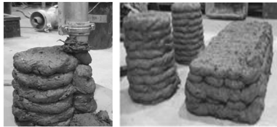
Fig. 6: 3D printed cob cylinders’ production from a robot arm.
